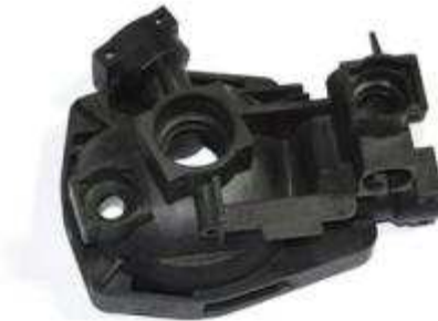
Injected with PA6
